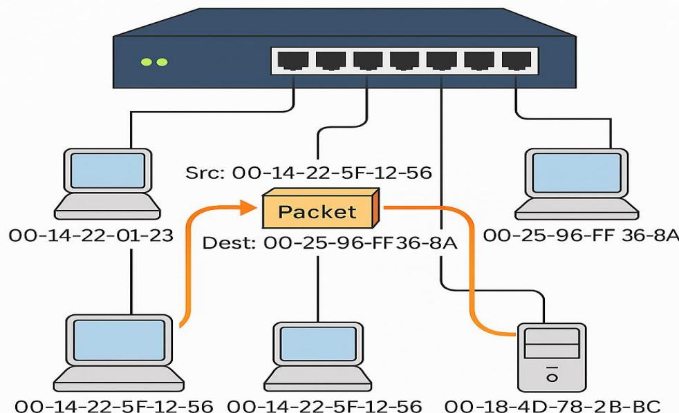
1.1-rasm. Switchning ishlash faoliyati
